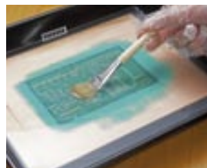
Developing the solder-resist mask
