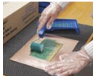
Applying the solder-resist lacquer
