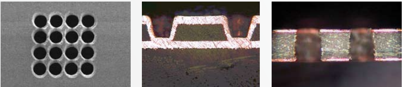
The LPKF ProtoLaser U produces excellent results when structuring 50 \mu\text{m} microvias or holes in HF material or FR4.
