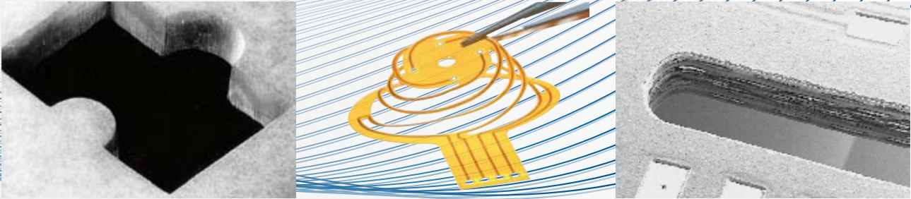
Precision cutting of assembled or unassembled materials – even with complex shapes: ceramics, polyimide and FR4.
