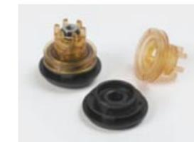
Valve parts – welded and unwelded
