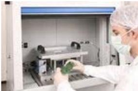
Using LPKF welding technology, a two-meter long welded seam was produced on a cartridge barely the size of a cellphone. During the welding process, the LQ-Vario MF monitors the whole procedure and records the parameters for seamless tracking & tracing.
