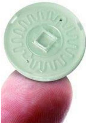
Laser plastic welding creates precisely welded seams in any pattern without harming the surrounding material. The integrity of the fine channel cross-sections is not affected. The laser also has built-in flexibility: if the weld contours must be modified, this can be simply done by loading the new layout data. Changing from one product to the next requires minimal time and effort.
