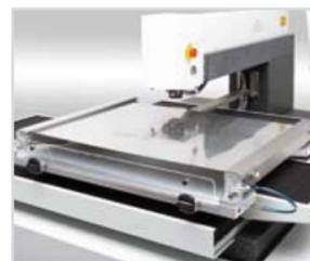
The LPKF SL AutoClamp S holds loose stencil sheets using a pneumatic uniform tensioning system.
